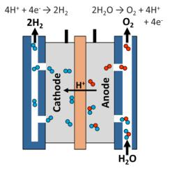
Water enters the system and reacts at the anode to form oxygen and positively charged Hydrogen ions (protons). Through an external circuit, electrons flow from the anode to the cathode while the Hydrogen ions selectively pass through the electrolyte in the PEM to the side of the cathode. At the cathode, the hydrogen ions combine with electrons from the external circuit to form hydrogen gas.
